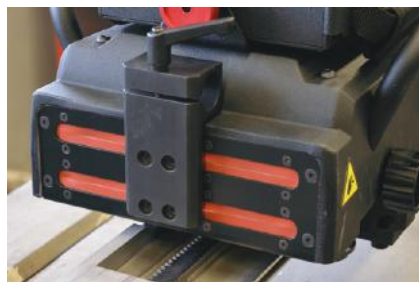
Silicone covers protect against dirt and spatter
