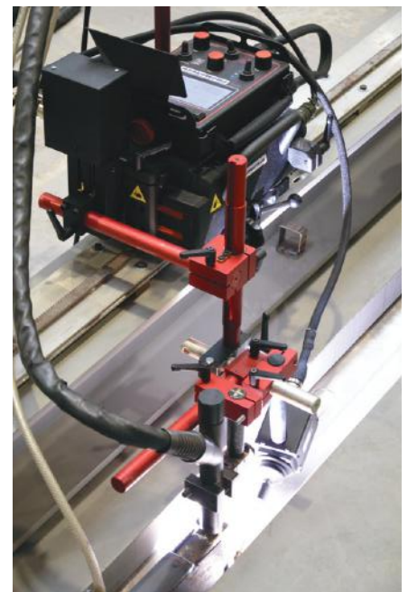
Seam tracking works with and without oscillation
