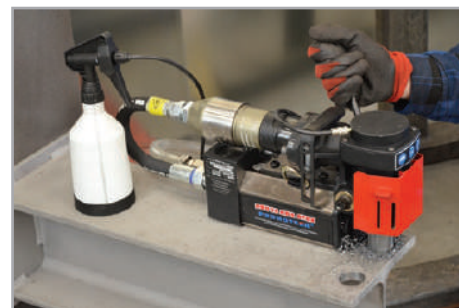
Through spindle cooling system
