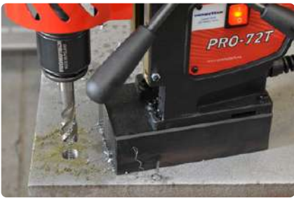
Tapping through holes up to M20
