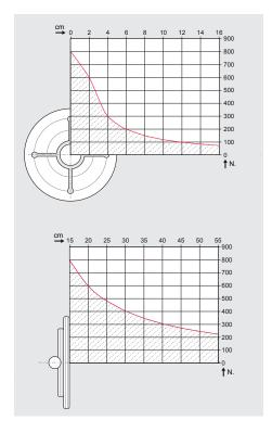
When choosing your positioner, please note the center of gravity of your workpiece incl. your tensioning device.
