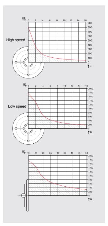
When choosing your positioner, please note the center of gravity of your workpiece incl. your tensioning device.
