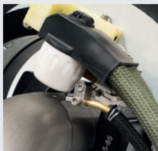
/ Wire feeding, torch bracket from 0 - 45° stepless swivelling
