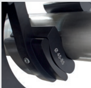
/ Reducer jaws depending on tube outer diameter
